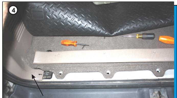
Position 5 bolt is located at very rear. Remove the plastic trim and rear panels, pull up carpet and remove the black square plug.
