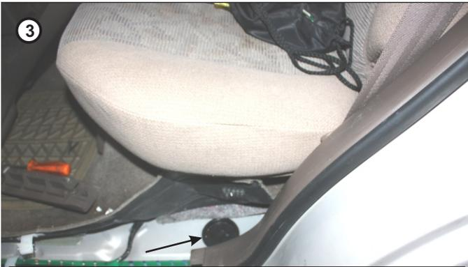
Position 4 bolt is located below the rear seat. Remove the plastic trim and panels, pull up carpet and remove the black round plug.
