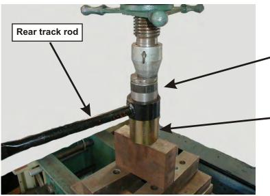
Inside Diameter of track rod is 1.417" (36mm). Push out old bushing with something smaller than 1.417".
