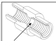
Bearing spacer I.D. has a 5/32" hex for tightening the first bolt.
