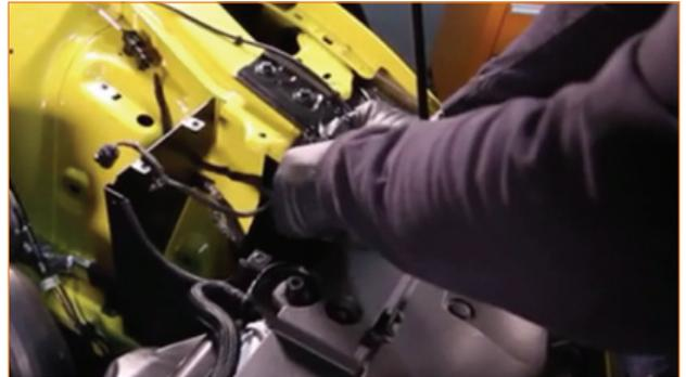
**25.** Insert the intake pipe and air filter into the engine bay. If the filter fitment is tight, turn the assembly slightly during install.
