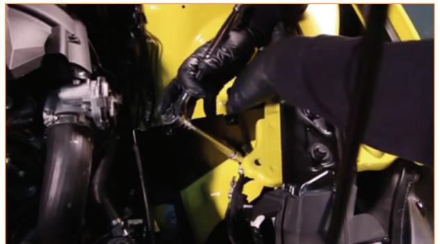
**18.** Install the two tree clips on the bottom, starting with the rearward tree clip.
