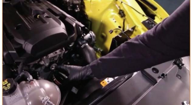
**24.** Remove the tree clip holding the wire harness to the body of your Mustang.
