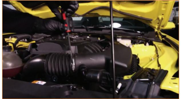
2. Disconnect the plug from the intake air temperature (IAT) sensor.
