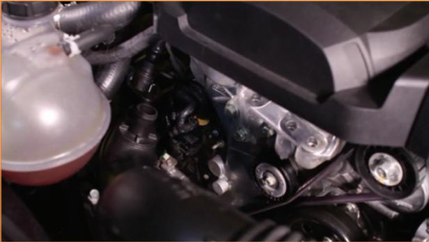
8. Loosen the worm-gear clamp connecting the intake tube to the turbo inlet. (flathead screwdriver)
