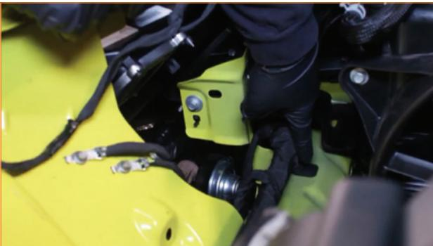
**15.** Loosen the 8mm top ground bolt but do not fully remove.
