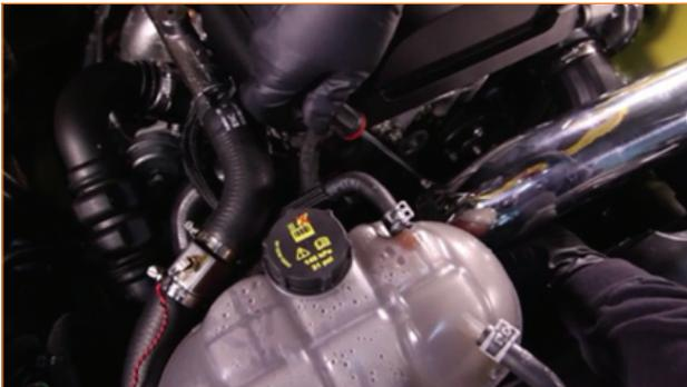
**28.** Fully tighten the T-bolt clamp that holds the inlet hose to the turbo. (10mm socket)
