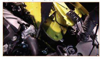
**17.** Make sure that the tab on the airbox falls in line with the ground bolt, and fully tighten the 8mm ground bolt.
