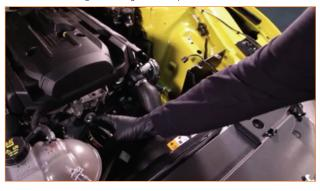
24. Remove the tree clip holding the wire harness to the body of your Mustang.
