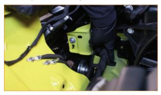
**15.** Loosen the 8mm top ground bolt but do not fully remove.
