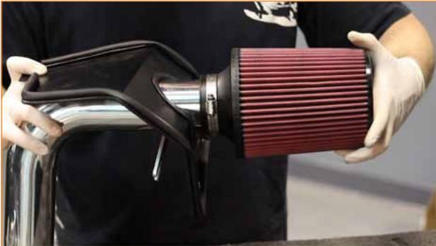
**4.** Tighten the clamp securing the air filter to the pipe, using a flathead screwdriver or 8mm socket.
