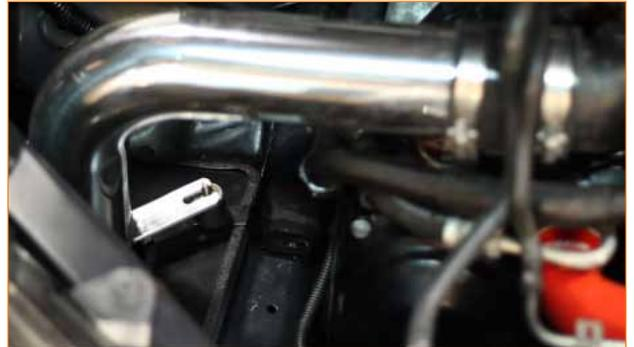
**10.** Using the 10mm bolt that was previously removed from the factory airbox, install the bolt through the heat shield bracket, securing it to the engine bay.
