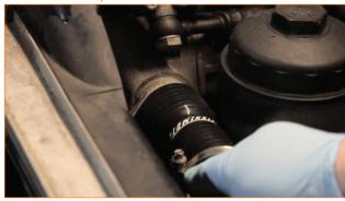
2. Install the new Mishimoto lower radiator hose, utilizing the OEM hose clamps again. Sliding the clamps onto the hose prior to installation is recommended due to the tight spaces.
