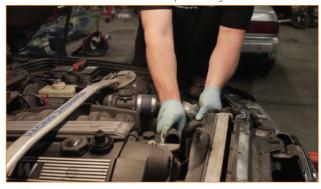
7. Remove the lower radiator hose. It is possible to do this from inside the engine bay. Using your flathead screwdriver, you will need to loosen the two hose clamps securing it. One is located on the lower side of the radiator, and the other on the front of the engine.
