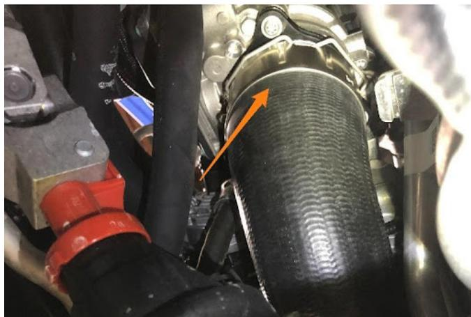
**25.** Remove the 3x T30 bolts from the throttle body adapter and remove the throttle body adapter from the vehicle.
