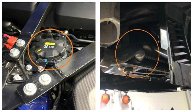
**09.** Remove the 4x 15mm bolts at 1x 13mm bolt holding the upper engine cross brace and V-brace then remove both braces from the vehicle. Remove engine cover from engine by pulling up. (Image on next page)
