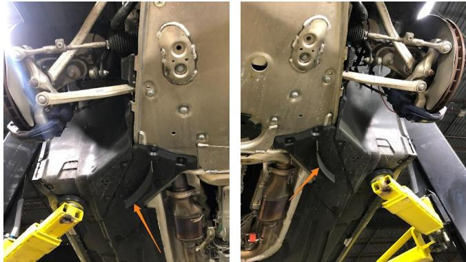
**05.** In each wheel well, remove the 2x (4x total) 10mm screws securing the large aluminum undertray to the wheel well liners.
