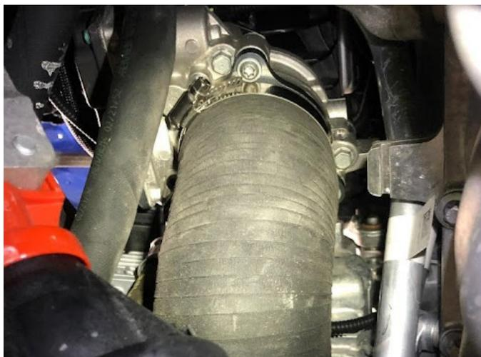
**33.** Install the front turbo adapter onto the outlet of the front turbo. There should be an audible click when the wire clip is fully seated.
