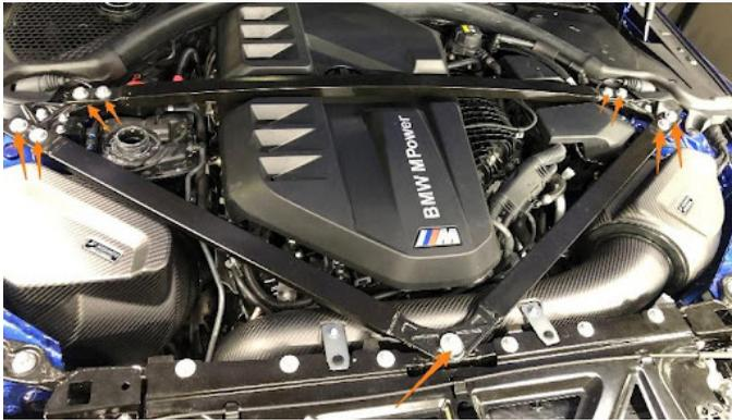
**10.** Remove the air intakes and air intake boxes. The factory intakes have a worm gear clamp at the end of the pipe near the air box and a quick disconnect near the turbos. Remove the 2x pop clips that attach the front turbo intake to the core support.
