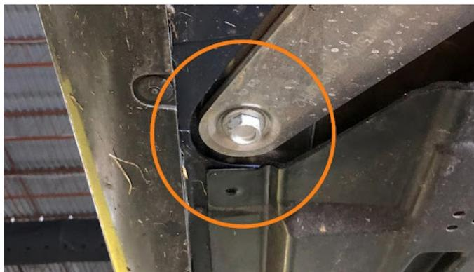
**07.** Remove the 11x 16mm bolts securing the large aluminum undertray to the vehicle. We suggest having a second person assist with removal as this undertray is quite large.
