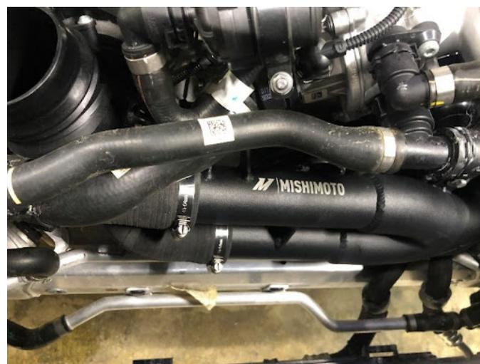
**39.** Reconnect and lock the electrical connectors for the intake temperature sensor and MAP sensor on the outlet of the Y-pipe.
