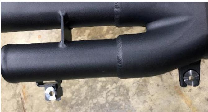
**30.** From underneath the vehicle, remove the spacer for the lower right side Y-pipe attachment point with a 17mm wrench or socket and replace with the included longer spacer. Torque to approx. 8 lb-ft.
