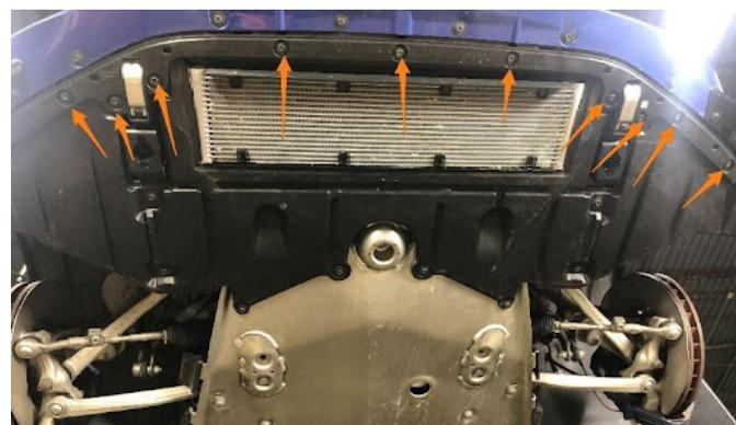
**03.** Remove the front and front-side plastic undertrays by removing all the 10mm screws holding it to the vehicle. There are 3x screws in each of the wheel wells holding the undertray to the bumper and wheel well liners. Remove undertrays from the vehicle.
