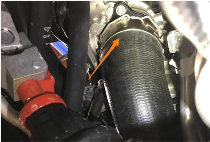
**29.** Install 4x grommets into the charge pipe. Remove the metal insert from each grommet, install the rubber piece into the charge pipe, and then reinstall the metal insert as shown.
