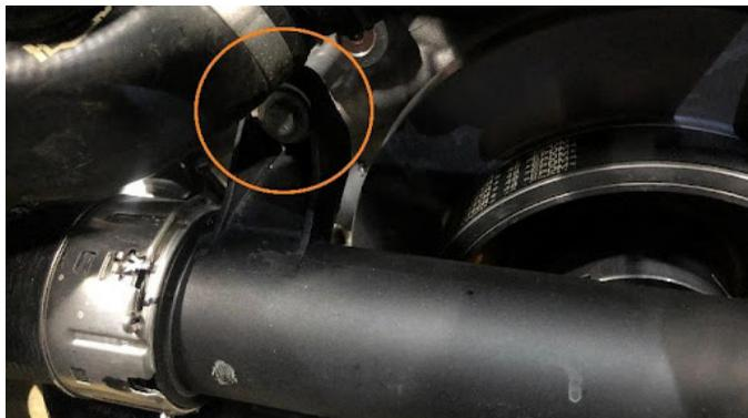
**21.** Locate the MAP sensor and temperature sensor in the outlet of the Y-pipe, next to the A/C compressor. Disconnect both electrical connectors. Moving the auxiliary water pump out of the way will help give access to the connectors. Both connectors have a white locking tab that must be pulled back to remove the connector.
