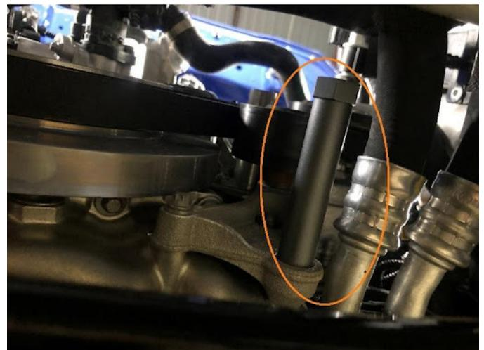
**31.** Install the included throttle body adapter onto the throttle body with the factory bolts. Torque bolts to approx. 8 N-m (6 lb-ft). The adapter should only be able to be installed in the correct orientation.
