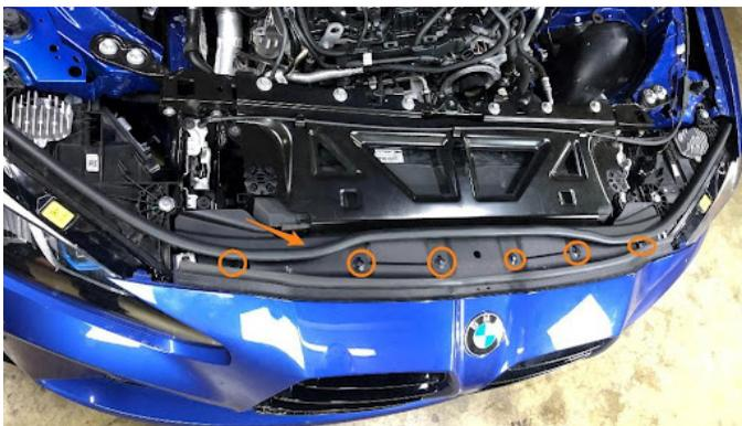
**12.** Remove the 6x 13mm bolts holding the radiator support panel. Remove the 4x silver T40 bolts, 5x black T30 bolts and move the hood latch cable out of the clips as shown.
