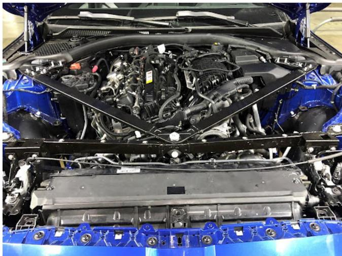
**46.** Reinstall the upper radiator support panel. First, reinstall the 4x pop clips. Then, install the 6x 13mm bolts, 4x T40 silver bolts, and 5x black T30 bolts hand tight. Then, torque the 3x black T30 bolts holding the bumper to the support panel to 4.6N-m.
