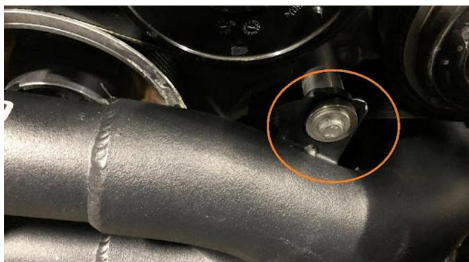
**37.** Install the 10mm bolt to secure the rear turbo pipe bracket. Tighten bolt to approx. 10 N-m (7 lb-ft).
