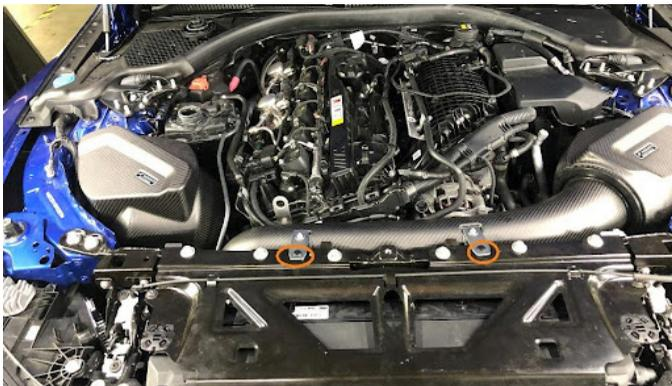
**11.** Remove the front hood seal by pulling up on the seal. Remove the 6x pop clips securing the front plastic panel to the vehicle and remove.
