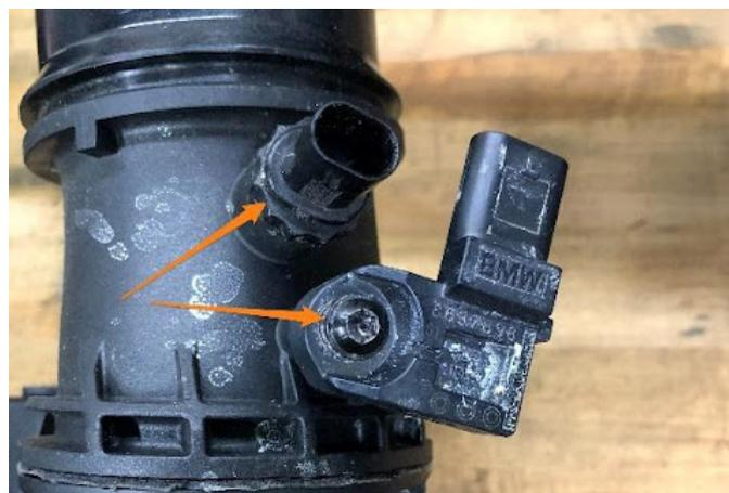
**27.** Install the temperature sensor in the Mishimoto Y-pipe. The sensor may need to be fully threaded in with a wrench but don't worry, it will not damage the threads. The sensor should be torqued to approx. 16 in-lbs.
