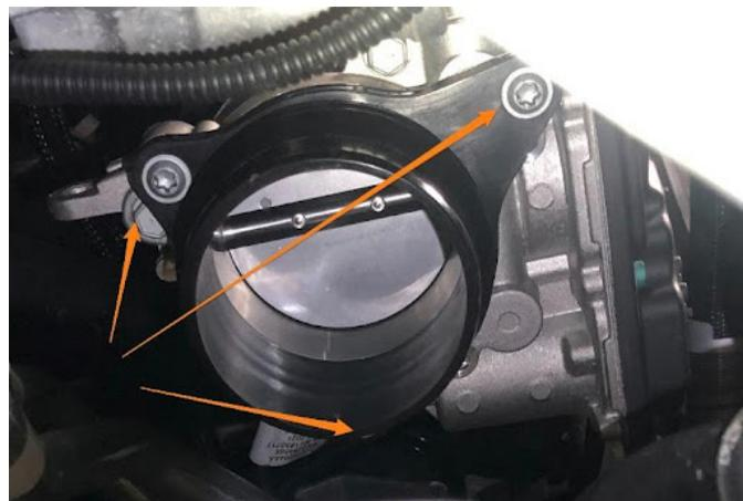
**26.** With a 17mm 12-point socket or wrench, remove the air temp sensor from the factory Y-pipe. Remove the T20 screw from the MAP sensor and remove the MAP sensor from the Y-pipe.
