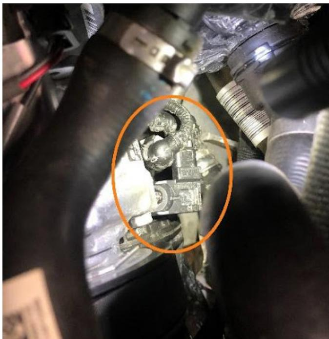
**22.** Remove the two inlet pipes and one outlet pipe from the large plastic Y-pipe by pulling the quick-disconnect clip back on both sides so that it locks into the "open position" then pull away from the pipe. The outlet pipe may be easier accessed from underneath the vehicle. Remove the Y-pipe from the vehicle.
