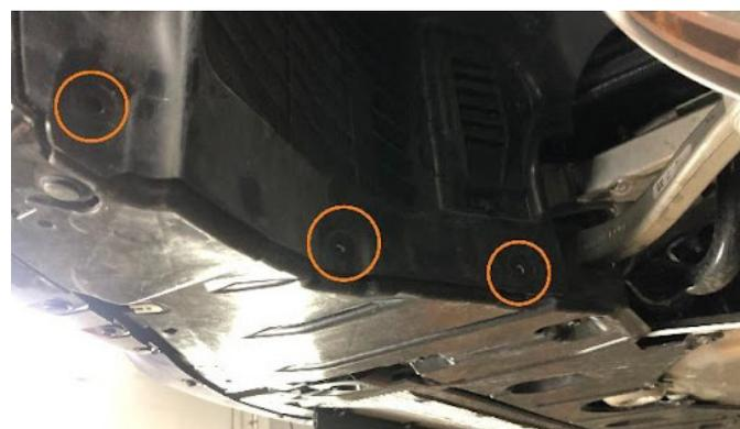
**04.** Remove the 10mm screws securing the rear undertrays to the vehicle. (Images on next page)
