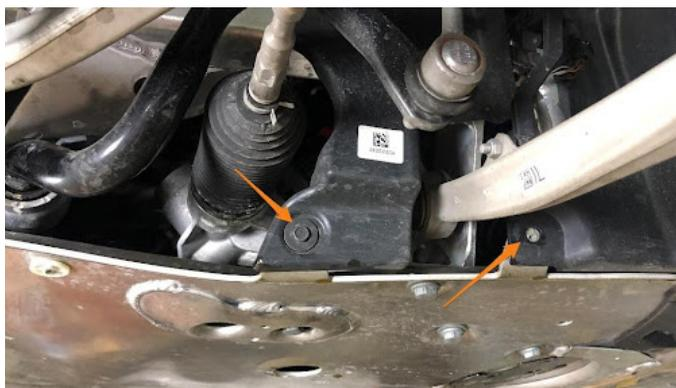
**06.** Remove the 2x 21mm bolts at the rear of the large aluminum undertray.
