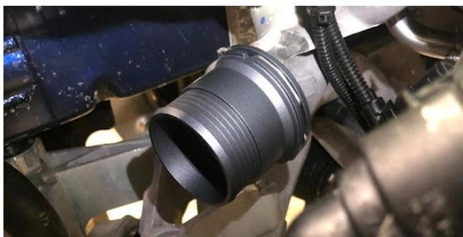
**34.** Install the last provided grommet into the bracket on the rear turbo pipe and install onto the rear turbo outlet. Make sure the bracket on the rear turbo pipe is on top of the bracket on the vehicle as shown. (Image on top right)
