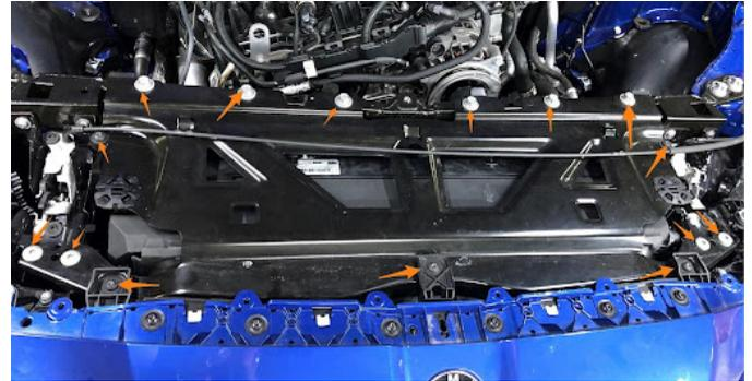
**13.** Remove the 4x pop clips behind the bumper that hold the radiator shroud to the radiator support panel. These clips may require you to pull back on the bumper for better access to the pop clips. Remove the radiator support panel from the vehicle.
