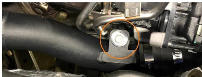
**38.** Adjust all 3x boots to ensure each boot is fully seated on each pipe. Then tighten each worm gear clamp to approx. 4 N-m (35 in-lbs) with an 8mm socket or flathead screwdriver. Make sure that each clamp is behind the bead roll on the pipes. The clamps and boots are not accessible in the engine bay once installed so it is critical that each clamp and boot is adjusted and properly tightened now.
