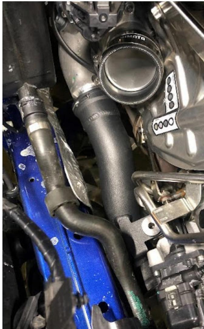
**35.** Install the front turbo boot onto the front turbo adapter. The slightly smaller end will go onto the front turbo adapter and the slightly larger end will go onto the lower inlet of the Y-pipe. Install the rear turbo boot onto the rear turbo pipe. The shorter end will go onto the rear turbo pipe and the longer end will go onto the Y-pipe. Refer to the parts diagram for further details. Install 2x 40-64mm worm gear clamps onto each boot, but do not tighten.
