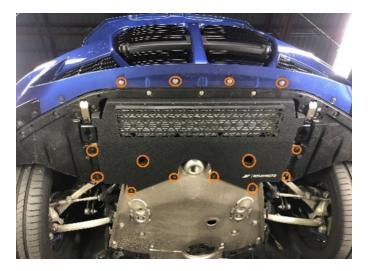
**05.** Remove 6x 10mm screws (per side) holding the side undertrays to the vehicle and remove from the vehicle to gain access to the auxiliary radiators. If you do not plan on draining the main cooling system, this is not necessary. We suggest draining the main cooling system as the throttle body coolant lines must be disconnected to remove the intake manifold/intercooler from the vehicle.
