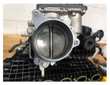
**26.** Remove the 3x 10mm bolts that hold the throttle body to the stock manifold. Make sure that both orange 0-Rings stay with the throttle body. (Image on top right)
