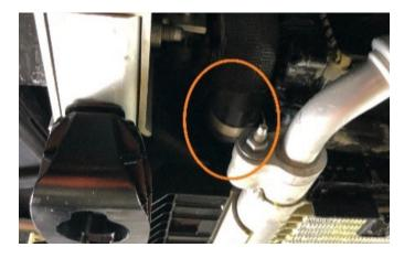
09. Remove 4x 15mm nuts securing the cross brace to the vehicle and remove. Remove the 4x 15mm nuts and 1x 13mm bolt securing the V-brace to the vehicle and remove. Remove the plastic engine cover by pulling up.
