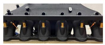
**47.** If you are using port injection, install the remaining fuel line into the fitting at the end of the fuel rail and tighten with a -6AN wrench.
