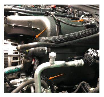
43. This manifold is capable of using both the factory rubber green O-rings or the included AFM gasket. We have provided the AFM gasket as it has thermal insulating properties to prevent heat transfer from the cylinder head to the intake manifold. At this time, remove the factory green o-rings from the factory manifold and install them onto the Mishimoto Manifold OR install the included gasket onto the pins on the Mishimoto manifold. USE THE O-RINGS OR THE GASKET BUT NOT BOTH!
