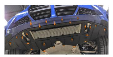
**02.** Drill out rivets to remove 2x oil cooler bash guards.
