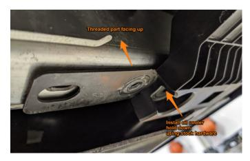
**07.** Bolt oil cooler bash guard, to bracket from step 6 using supplied M6 bolt.
