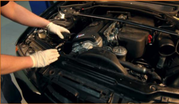
8. Disconnect the plug on the stock fan shroud.
