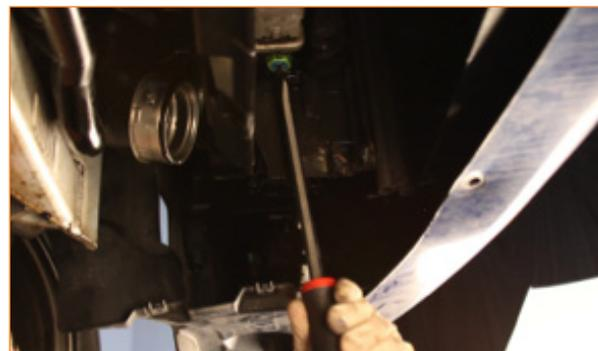
6. Once the fluid has completely drained, reinstall the drain plug. (flathead screwdriver)
