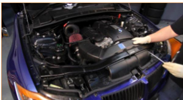
2. Loosen the bleeder on the coolant reservoir. (flathead screwdriver)
