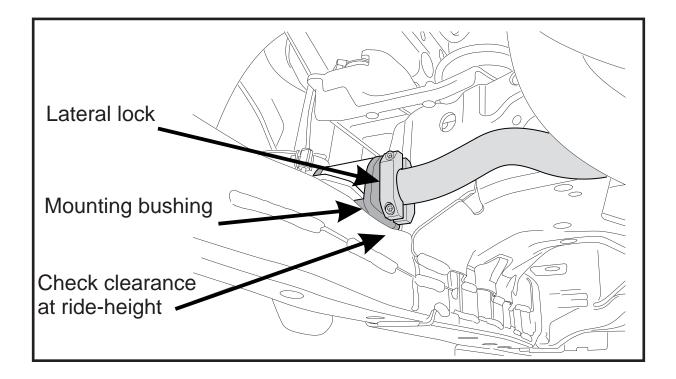
Confirm your Swaybar is central with links attached - this is best performed at ride-height.
