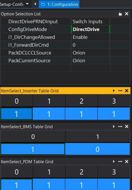
The screenshot shows the 'Setup-ConfigOptions' group with the '1: Configuration' tab selected. It displays an 'Option Selection List' with the following settings:
