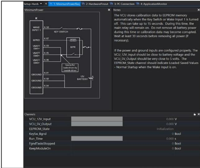
Select the MinimumPowerReq tab which includes an example wiring schematic and general information about power distribution. Use the Hardware Pinout and the Minimum Power schematic shown to build a test bench harness that can be powered from a 12V bench top power supply.
