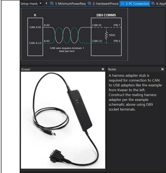
Select the PC Connection tab. Assemble and add a PC communications stub to your harness. Use the example schematic for reference. The VCU300 communicates with your PC via a CAN to USB adapter. If you do not have experience assembling harnesses for use in vehicle networks, please seek help from an experienced automotive harness builder. The VCU300 functions as a CAN network data hub. Proper network wiring is critical for performance and safety.
