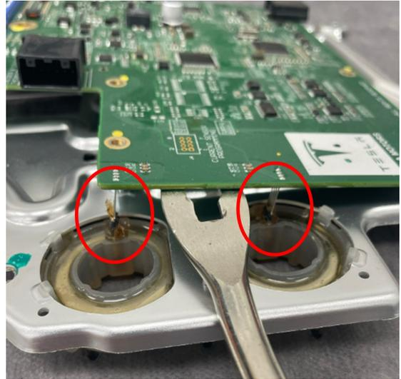
13. Remove blue connector position assurance lock from brown main connector. This can be achieved by gently prying the snap hooks on the connector inward with a small screwdriver while simultaneously prying upward on the blue lock. Work you way around one lock at a time. Care must be taken or the small fragile snap hooks can be broken. Once all 4 locks are released the blue CPA lock and brown connector can be removed from the factory inverter board and set aside.
