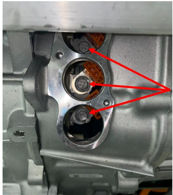
4. Remove inverter housing screws with 8mm socket (10 screws). Support inverter housing after all screws have been removed as there are two wired connections that must be released internally before the inverter is free. If the inverter is not fully supported damage to the inverter may result.
