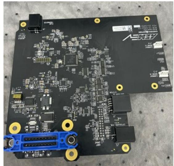
16. Place the AEM inverter board onto the metal EMI chassis as shown. Make sure to position the current sensors into the small cavities that were created by removing the ultra viscous clearsealing compound. Some resistance is expected but if the current sensors on the new board feel like they are binding up the holes in the compound may need to be further enlarged. The compound will compress a fair amount as it is relatively soft.
