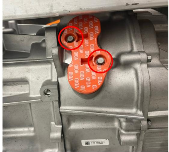
3. Remove the phase screws from the internal inverter cables via the access ports that are now accessible from the removal of the cover. (3 screws) will require a 10mm socket.
