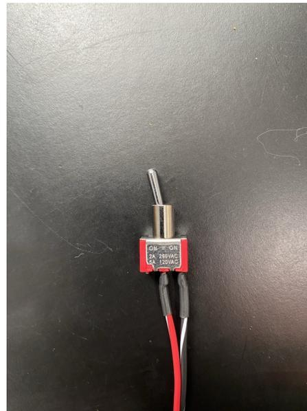
GUI MODE Point switch towards the Red with White Stripe wire for GUI mode.
