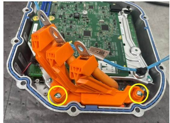
7. Pull the phase cable housing free of the inverter case by bending the phase cables inward toward the board. Then slide each of the phase cables out of the front of the orange housing.
