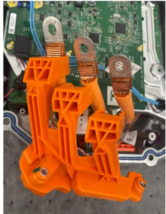
8. Using a panel removal tool, pop the 3 cable retention clips (yellow circles) free from the metal EMI chassis. At this time the 3 connectors (red circles) can be unplugged. Remove the blue harness from the assembly and set aside.
