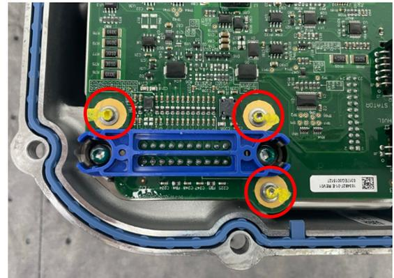
10. Remove the 5 screws from the metal EMI chassis that hold the inverter board in place using T20. Gently remove factory inverter board and chassis from housing assembly by sliding past phase cables. Set housing aside.
