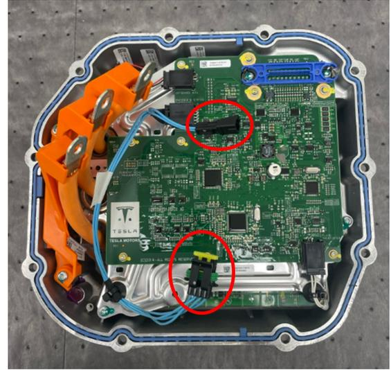
6. Remove the 2 screws (T20) that hold the orange phase cable housing to the inverter case.
