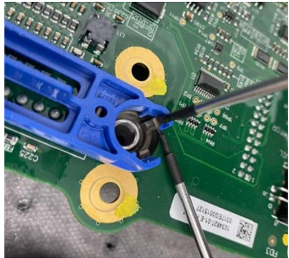
14. Using a small flat screwdriver or pick tool “dig” the ultra viscous clearsealing compound out of the cavity where the current sensors previously occupied. Take care not to damage the current sensor rings that are still embedded in the compound. Dig out a generous cavity and then use compressed air to blow any residual “crumbs” of the material free of the assembly. The image shows an enlarged cavity on the top and on the bottom is prior to compound removal.
