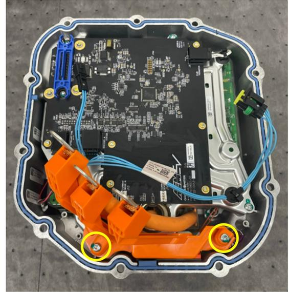
23. The inverter assembly is now ready to be reinstalled in the drive unit. Position the inverter near the drive unit and reconnect the encoder and temperature connectors. Make sure they are fully connected.
