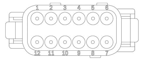
Mini Master BMS Connections as viewed from the wire entry side of the Connector **Unsealed Satellite BMS**
