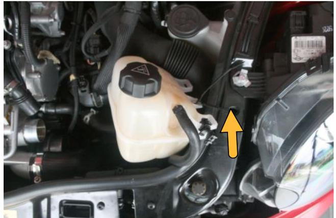
Unclip the electrical connector from the diverter valve (
