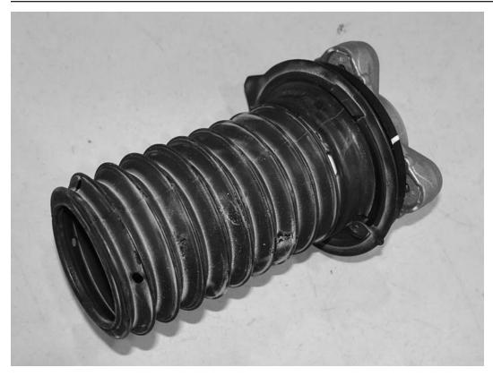
23) Install the stock shock bellows onto the top shock bearing with the Dinan bump stop still inside.
