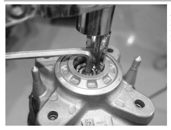
19) Using a commercially available 18mm shock socket and a 6mm allen wrench, loosen and remove the nut that holds the upper shock mount to the shock. Remove the upper shock mount from the shock. For safety purposes, release the tension on the spring.
