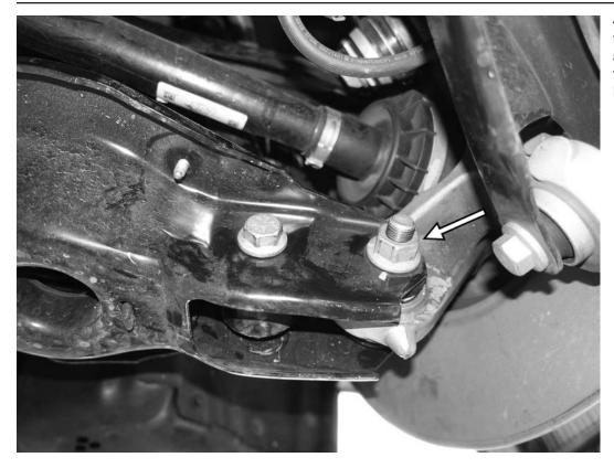
47) While holding the back side of the E20 external torx bolt, loosen and remove the 21mm nut from the front side of the lower control arm. Do not remove the bolt yet.
