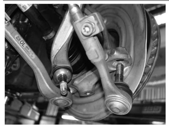
13) Separate the control arms and tie rod from the upright so that the upright, brake rotor, and shock assembly is only held in place by the upper nuts.
