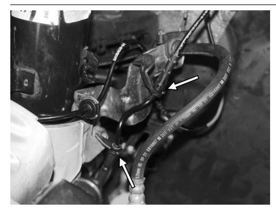
3) Follow the wiring harness to the brake pad wear indicator at the caliper. Separate the harness from the two mounting tabs on the bracket mounted to the back side of the shock.
