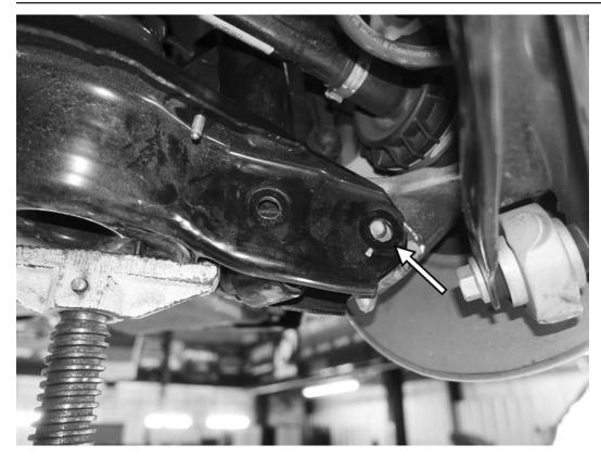
61) Use a pole jack or transmission jack to raise the lower control arm until the outer E20 external torx bolt to the rear upright can be installed freely from the back side of the control arm. Do not hammer or force the bolt in place. BMW recommends replacing this bolt every time it is used.
