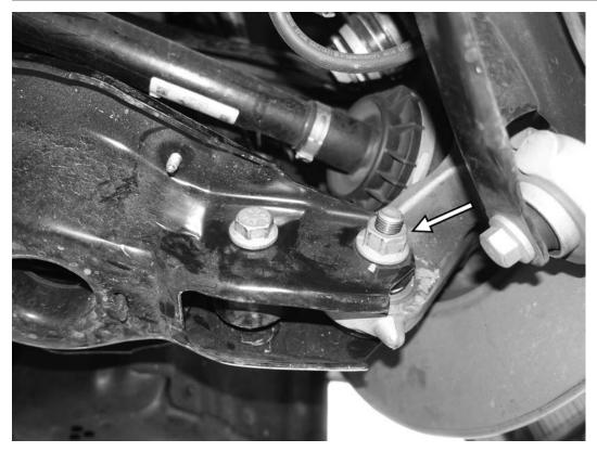
63) Install the 21mm nut on the front side of the bolt holding the lower control arm to the upright. While counterholding the E20 bolt, tighten the 21mm nut to 165Nm (121 ft-lbs). Once torqued, tighten the 21mm nut an additional 90°. BMW recommends replacing this nut every time it is used.
