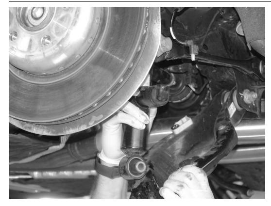
53) Pull down on the lower control arm while holding the rear shock, and then remove the rear shock from the car.
