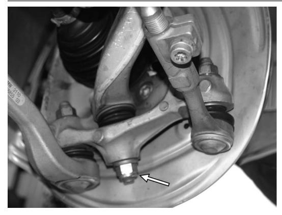
33) Begin to reinstall the arms into the bottom of the upright. Install the middle control arm first, installing and tightening the 21mm nut to 175Nm (129 ft-lbs). Use a T40 socket to prevent the joint from rotating while tightening. BMW recommends replacing this nut every time it is used.
