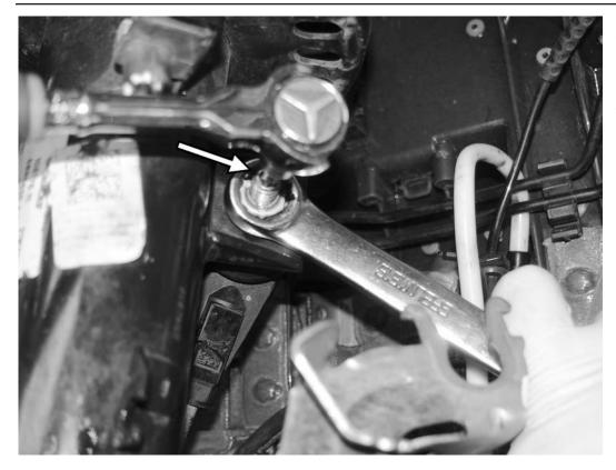
11) Use a 16mm combination wrench and a T30 socket to remove the nut holding the sway bar endlink to the shock. Hold the endlink with the T30 in the middle of the shaft from the endlink, while loosening the 16mm nut. Separate the end-link from the shock once the nut is removed.
