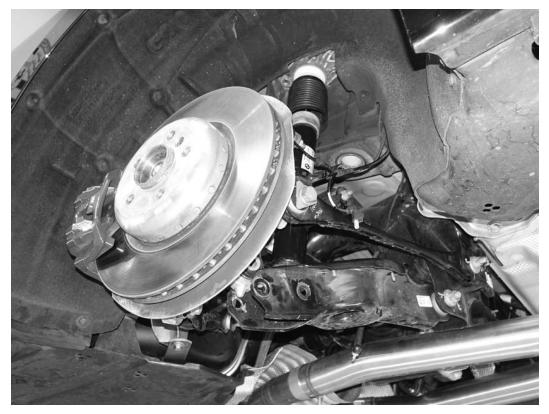
57) After pulling down the rear lower control arm, restall the shock in the car.
