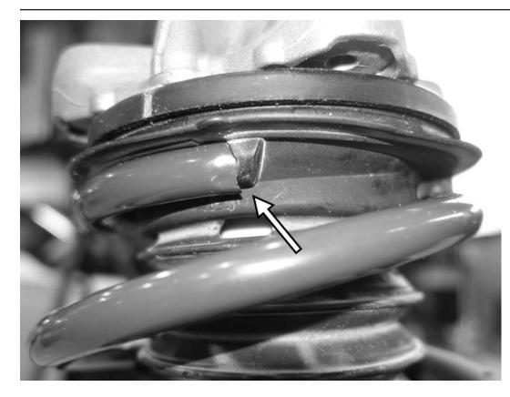
27) Release the tension on the Dinan spring. Ensure the top of the Dinan spring is sitting next to the tab on the bottom of the shock bearing.
