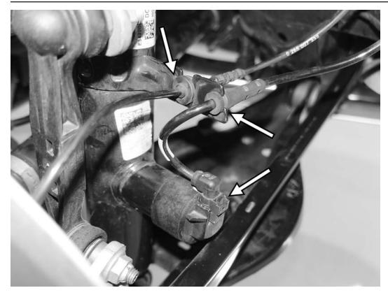
51) If installing the Dinan handling kit, perform steps 51-58., otherwise skip to step 59. Separate the rear ABS sensor harness from the bracket on the back of the rear shock. Separate the rear shock wiring harness from the same bracket, and then unplug the harness from the back of the shock.
