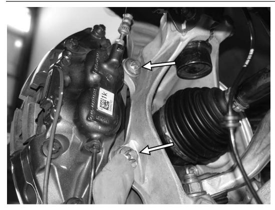
9) Remove the two E16 external torx bolts holding the brake caliper to the upright.
