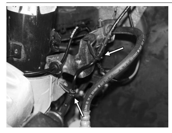
41) Reinstall the brake pad wear indicator harness from the brake caliper. Connect the harness to the two mounting tabs on the bracket mounted to the back side of the shock. Route the harness in the same path that it was routed stock.
