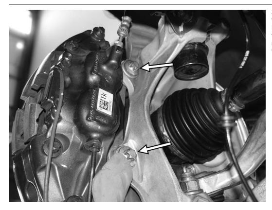
37) Reinstall the brake caliper to the back of the upright with the two E16 screws. Tighten the two screws to 130Nm (96 ft-lbs). BMW recommends replacing these screws every time they are used.
