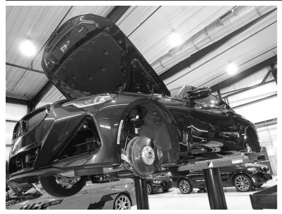
1) Place the vehicle on a lift or securely on jackstands and remove twenty lug bolts and all four wheels with a 17mm socket.
