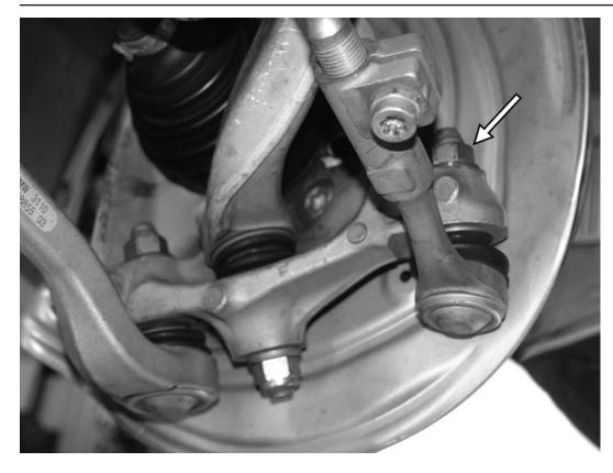
35) Install the tie rod arm next, installing and tightening the 21mm nut to 165Nm (121 ft-lbs). Use a T40 socket to prevent the joint from rotating while tightening. BMW recommends replacing this nut every time it is used.
