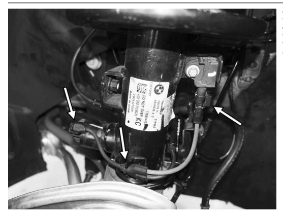
43) Reinstall the wiring harness to the front shock. Place the grommet on the harness into the bracket on the shock, and then reconnect the two electrical connectors on the front and the back of the shock.
