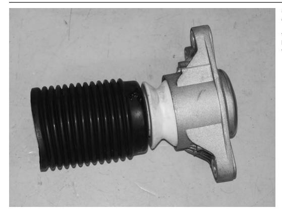
55) Remove the stock bump stop and dust cover from the rear shock. Install the Dinan bump stop into the top shock mount. A thin coating of lubricant may be necessary to push the bump stop into the mount.
