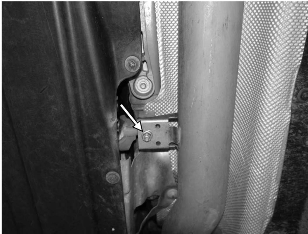
13) With an assistant holding the rear muffler of the car, remove the previously loosened 13mm nut from the front hanger of the exhaust. Separate and lower the exhaust from downpipe, and remove the full exhaust system from the car.
