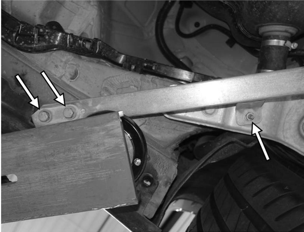
27) Install the two 13mm screws from the front side of the chassis stiffening brace, and then install the one 13mm nut from the middle bracket on the braces. Repeat these steps on the right side side of the car. Tighten the six 13mm screws on the chassis stiffening brace to 100Nm (74 ft-lbs). Then tighten the screws an additional 90°. Tighten the two 13mm nuts on the brace to 28Nm (21 ft-lbs). BMW recommends replacing these screws and nuts every time they are used.
