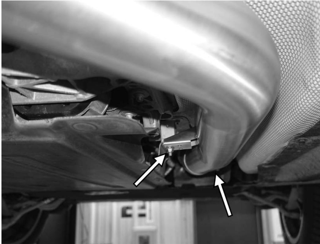
29) Working from the front of the car to the back, tighten the 13mm nut on the front exhaust hanger to 19Nm (14 ft-lbs). Then, tighten the front clamp to the downpipe to 45Nm (33 ft-lbs).
