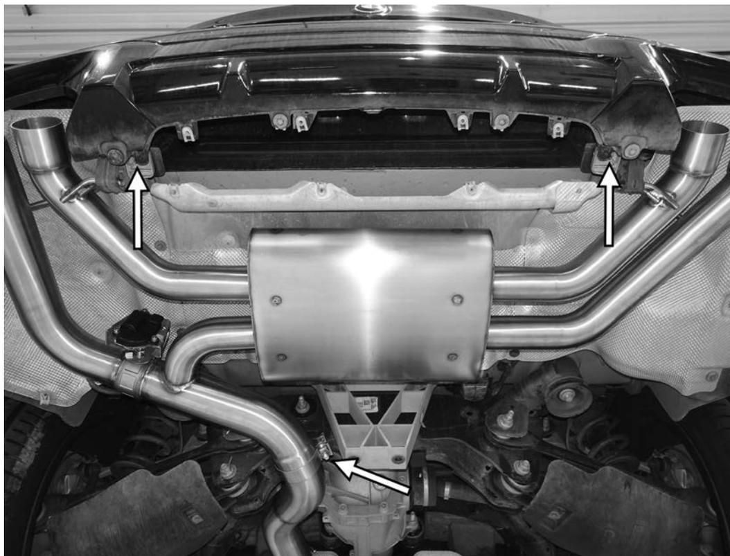
21) Install the rear muffler with the second of the two bigger clamps and the two 13mm nuts that held the factory rear exhaust hangers in place. The system should not be fully tightened yet, but should be secure enough to stay in the same location.
