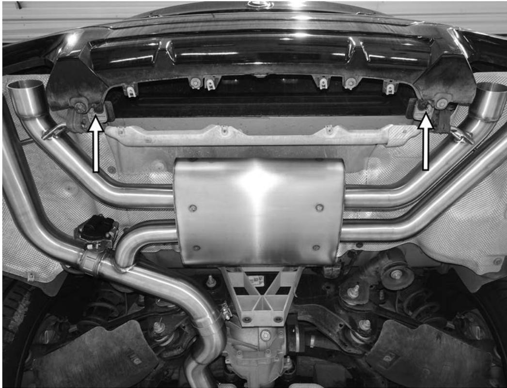
31) Once adjusted, fully tighten the two 13mm nuts on the rear factory hangers on the back of the Dinan rear muffler. Tighten the nuts to 19Nm (14 ft-lbs). BMW recommends replacing these nuts every time they are used.
