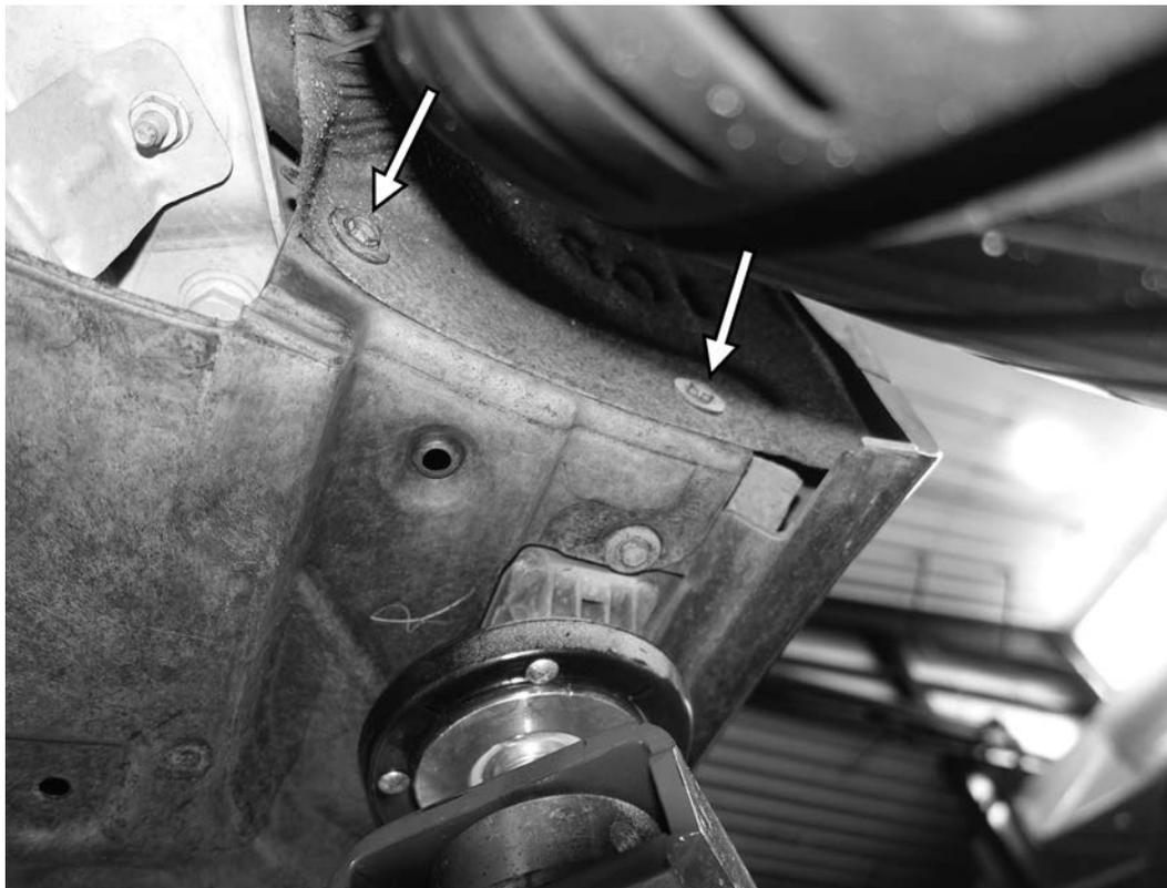
35) Reinstall the two 10mm screws holding the underbody panel and the wheel well liner together. Tighten these to 2.6Nm (23 in-lbs). Repeat this process on the other side of the car.
