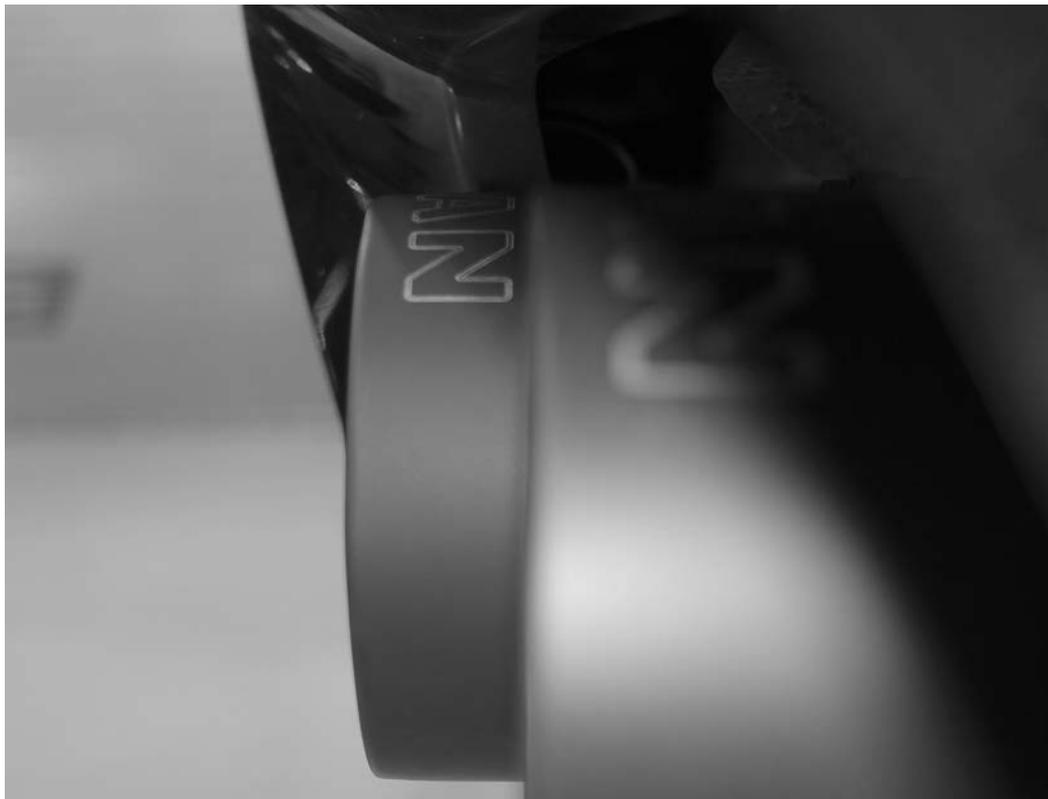
25) For reference, the outer Dinan tips should begin at the top of the Dinan letters of the inner tip. This is not a final adjustment, so do not tighten the clamps on the tips yet.
