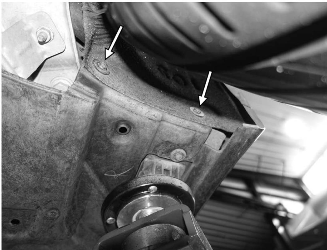
3) From the front side of the rear wheel well, remove the two 10mm screws holding the rear wheel well liner and middle underbody panels. Repeat this step on the left side of the car.
