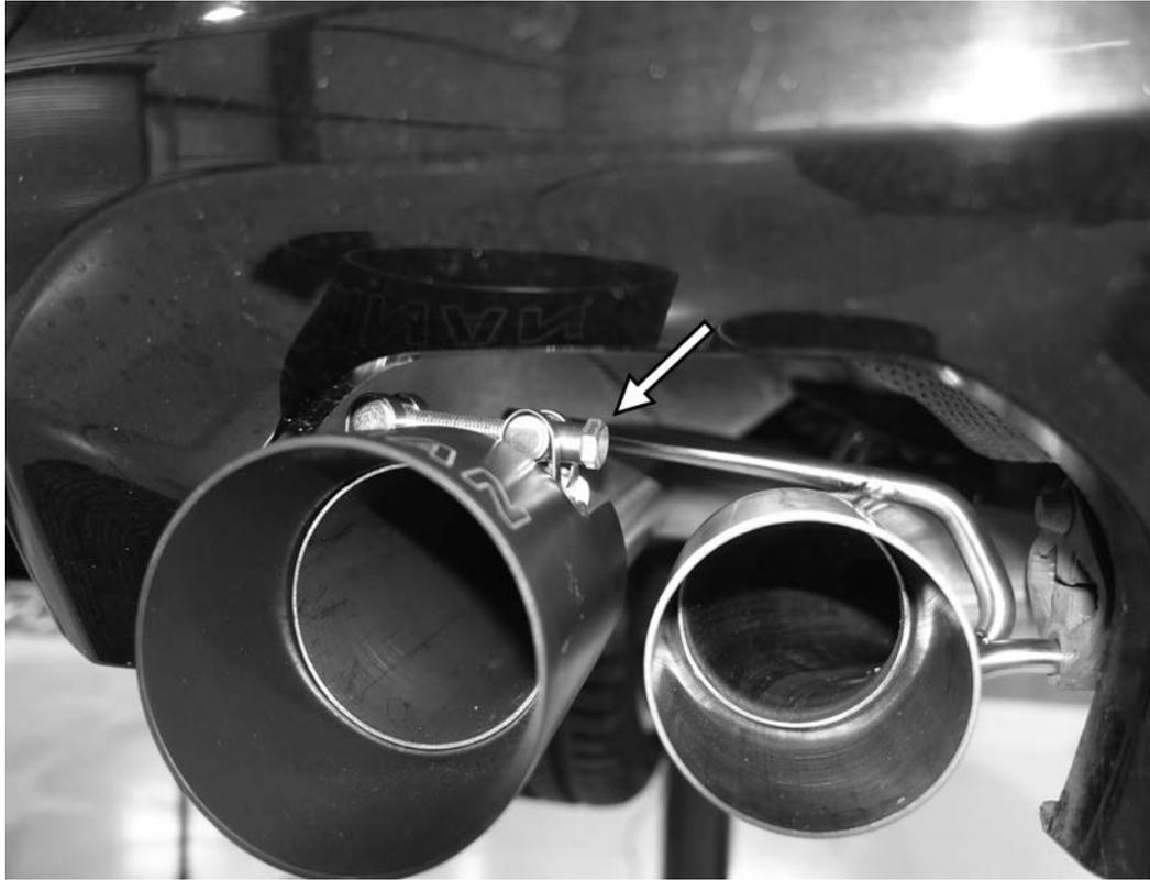
23) The outer left exhaust pipe is a larger diameter than the other three. Find the one Dinan exhaust tip that has a slightly larger inlet and install it on the larger exhaust pipe with the one larger exhaust tip clamp. Tighten the tip somewhat, but leave loose enough to be manipulated.
