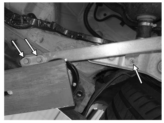
7) Remove the two 13mm screws from the front side of the chassis stiffening brace, and then removed the one 13mm nut from the middle bracket on the braces. Repeat these steps on the right side side of the car. Remove the two rear 13mm screws previously loosened from the rear vertical brace, and remove the stiffening braces from the car.
