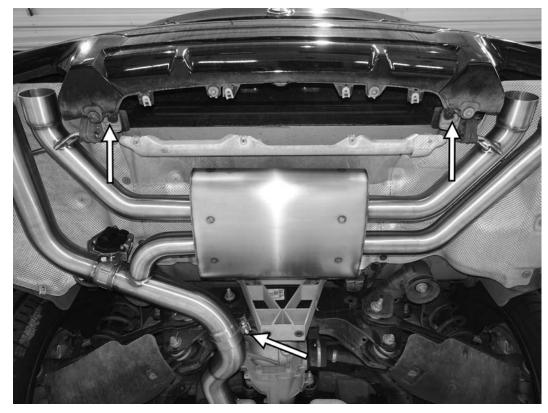
21) Install the rear muffler with the second of the two bigger clamps and the two 13mm nuts that held the factory rear exhaust hangers in place. The system should not be fully tightened yet, but should be secure enough to stay in the same location.
