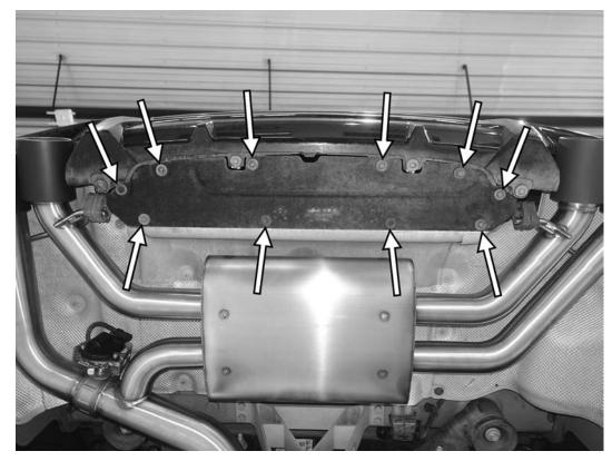
33) Reinstall the panel that goes between the bottom of the rear bumper and the exhaust heat shield. Secure the panel with the ten 10mm screws, and tighten the screws to 2.6Nm (23 in-lbs).
