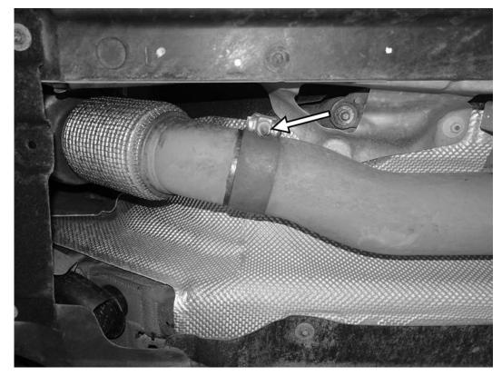
11) Loosen the 13mm nut on the clamp holding the front side of the exhaust to the downpipe. Separate the clamp from the clamp from the exhaust.
