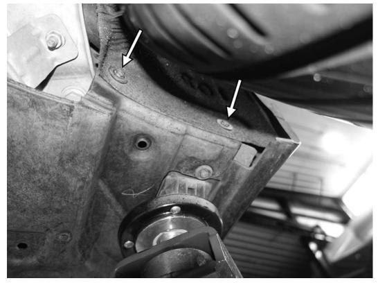
3) From the front side of the rear wheel well, remove the two 10mm screws holding the rear wheel well liner and middle underbody panels. Repeat this step on the left side of the car.
