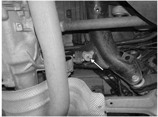
9) Remove the 13mm nut holding the right middle exhaust hanger to the rear subframe, just in front of the rear axle shafts. Repeat this set on the corresponding hanger on the left side of the car.
