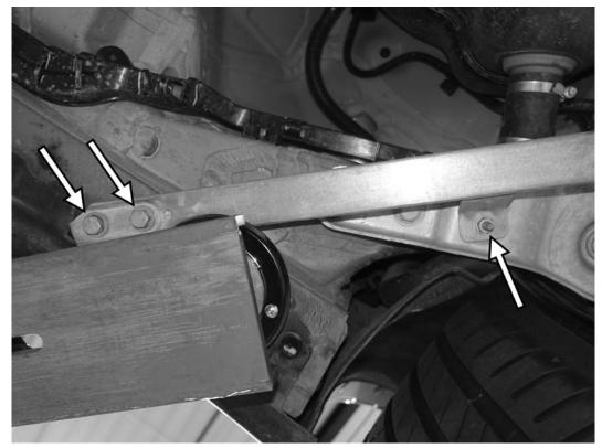
27) Install the two 13mm screws from the front side of the chassis stiffening brace, and then install the one 13mm nut from the middle bracket on the braces. Repeat these steps on the right side side of the car. Tighten the six 13mm screws on the chassis stiffening brace to 100Nm (74 ft-lbs). Then tighten the screws an additional 90°. Tighten the two 13mm nuts on the brace to 28Nm (21 ft-lbs). BMW recommends replacing these screws and nuts every time they are used.
