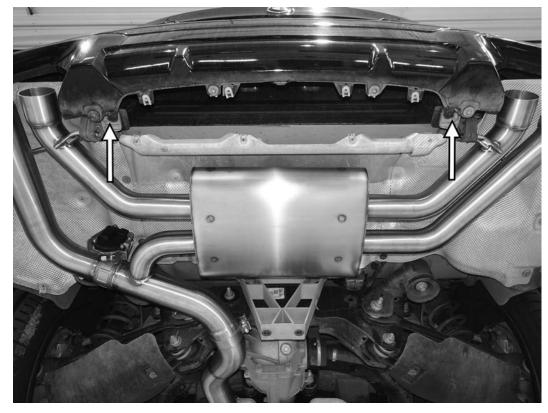
31) Once adjusted, fully tighten the two 13mm nuts on the rear factory hangers on the back of the Dinan rear muffler. Tighten the nuts to 19Nm (14 ft-lbs). BMW recommends replacing these nuts every time they are used.
