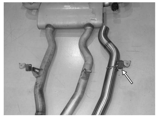
15) Place the Dinan exhaust midsection next to the left side of the factory exhaust. Swap the factory exhaust hanger from the left side of the factory exhaust to the hanger on the Dinan midsection. 16) With one of the two bigger supplied clamps, install the Dinan midsection to the back of the Dinan front section. Install the 13mm nut to secure the factory hanger to the chassis. Tighten the 15mm nut on the clamp enough to where the exhaust can still be manipulated, but not fully tightened.
