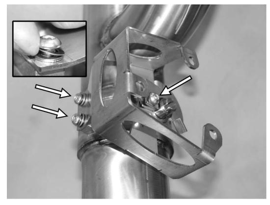
17) Install the bracket to the Dinan exhaust valve with the three 4mm allen screws, three flat washers, and three spring washers. The flat washer will be closest to the bracket, then the spring washer, then the screw. Tighten the 4mm allen screws to 14Nm (10 ft-lbs).
