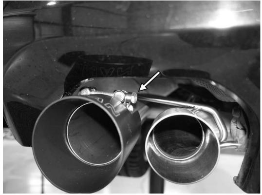
23) The outer left exhaust pipe is a larger diameter than the other three. Find the one Dinan exhaust tip that has a slightly larger inlet and install it on the larger exhaust pipe with the one larger exhaust tip clamp. Tighten the tip somewhat, but leave loose enough to be manipulated.
