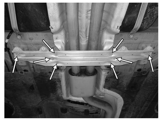
5) Remove the eight E10 external torx screws from the crossbrace at the center of the car. Remove the crossbrace from the car.
