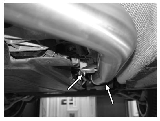
29) Working from the front of the car to the back, tighten the 13mm nut on the front exhaust hanger to 19Nm (14 ft-lbs). Then, tighten the front clamp to the downpipe to 45Nm (33 ft-lbs).
