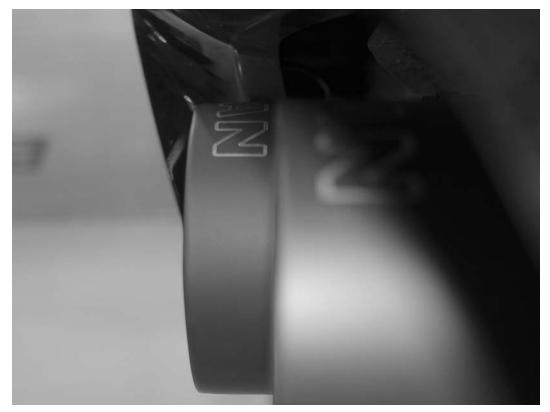
25) For reference, the outer Dinan tips should begin at the top of the Dinan letters of the inner tip. This is not a final adjustment, so do not tighten the clamps on the tips yet.
