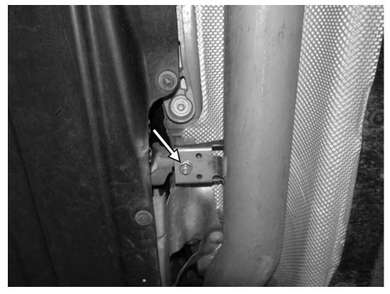
13) With an assistant holding the rear muffler of the car, remove the previously loosened 13mm nut from the front hanger of the exhaust. Separate and lower the exhaust from downpipe, and remove the full exhaust system from the car.
