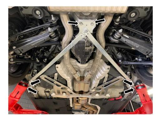
2) Remove these 6 bolts from the V-brace and remove the brace.
