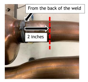
2) Cut the pipes per the 2 marks you've made. Your exhaust should look like the picture below.
