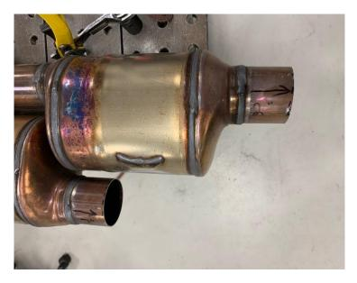
3) Cut the bracket that holds both catalytic converters together off. It is recommended to use a cutoff wheel.
