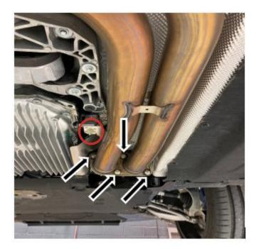
3) If you have a stock exhaust system, once the exhaust is removed, cut the stock exhaust at the factory cut points.
