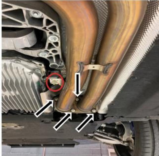
3) If you have a stock exhaust system, once the exhaust is removed, cut the stock exhaust at the factory cut points.
