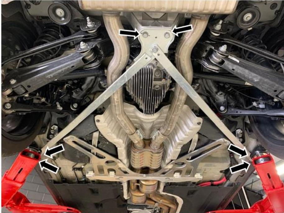
3) Remove these 12 bolts from the center brace and remove the brace.
