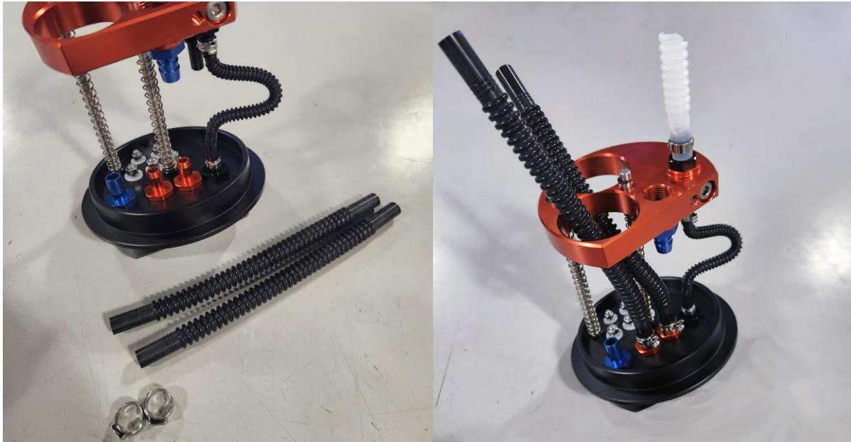
6 – Locate the larger 8" (200mm) x 3/8" (10mm) convoluted tube and two of the 13mm pinch clamps. Install the hose on the two blue barb fittings on the bottom side of the module tophat and top of the orange pump holder. Secure them with the clamps.
