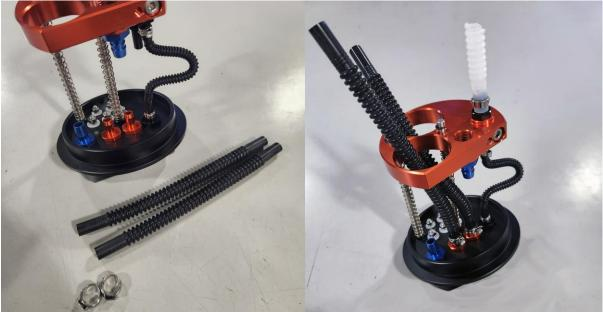
$6 - Locate the larger 8'' (200mm) \times 3/8'' (10mm) convoluted tube and two of the 13mm pinch clamps. Install the hose on the two blue barb fittings on the bottom side of the module tophat and top of the orange pump holder. Secure them with the clamps.$
