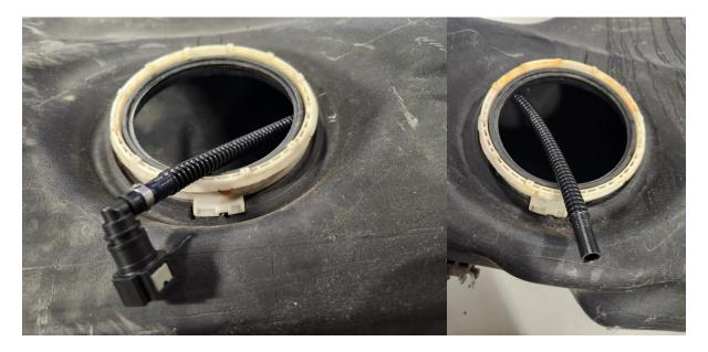
18– Remove the OEM drivers side fuel level sensor hanger, the E36 and E46 hangers are slightly different. Slash cut the end of the new venturi suction hose at an angle, so it matches the OEM venturi pickup as shown. Using the supplied zip ties attach the new venturi suction hose to the OEM hanger so it is as close as possible to the bottom of the fuel tank, this will allow you to get the highest capacity from your fuel tank as possible.
