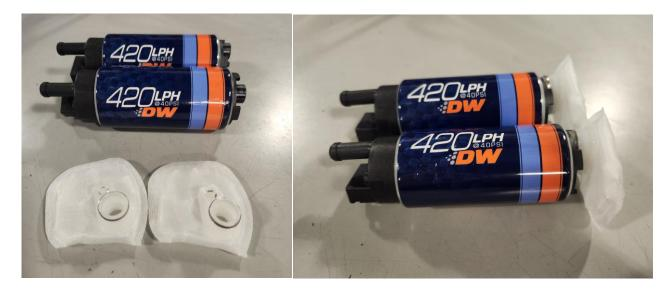
12 – Slide the pumps into the bucket assembly, double check that the filter socks did not knock the rubber check valves from Step 2 out of position. Slide the X-series module tophat and pump holder assembly over the pumps and down into the bucket, secure it in place with the three M6 bolts.
