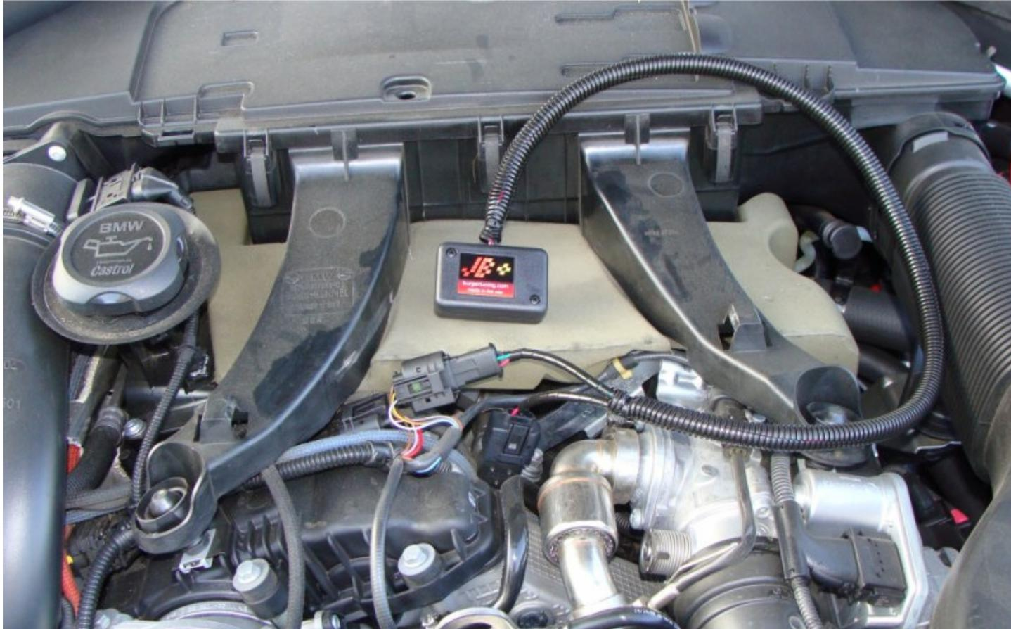
Once connected route the JBD harness to the driver side of the engine bay as shown and secure with a zip tie, twist tie, or simply shove it in a corner.
